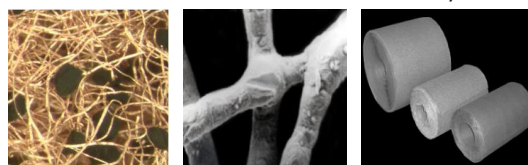
Figure 3. Left: Optical micrograph of Cu MFEC for FTS. Middle: SEM micrograph of a sintered fiber junction. Right: Rolls of Microfibrus Media
